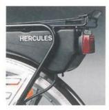
Good position: the tank has a volume of 1.5 l. It will carry you over a distance of more than 100 km – without using your legs.
